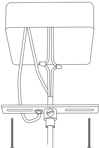
**9** Install frame with allen set screw onto socket lamp.
